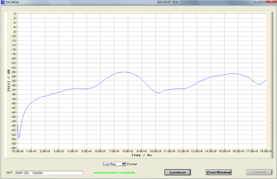
Fig. 6-8 Graphical display of the reflection measurement results
